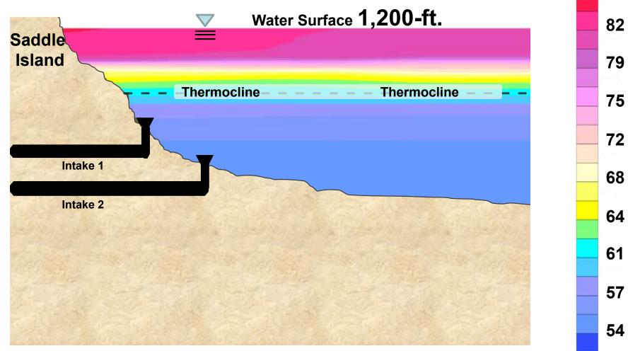
Intakes below the thermocline substantially avoid the impacts of poor water quality effects from Las Vegas Wash discharges
