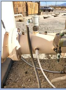
Cr6 Reduction Calibration Test (0.5 ppm Sn & 0.5 ppm Cl2)
